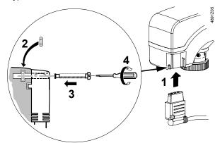
The cable connector snaps into position, but can be additionally secured with the retaining screw.
